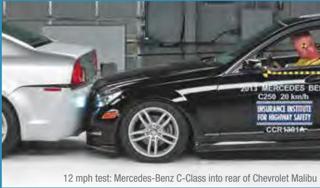
12 mph test: Mercedes-Benz C-Class into rear of Chevrolet Malibu
