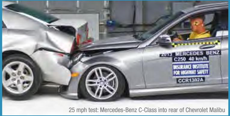
25 mph test: Mercedes-Benz C-Class into rear of Chevrolet Malibu
